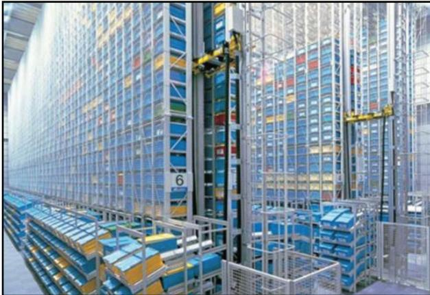
Figure 9: Automated Storage & Retrieval Systems (ASRS)
